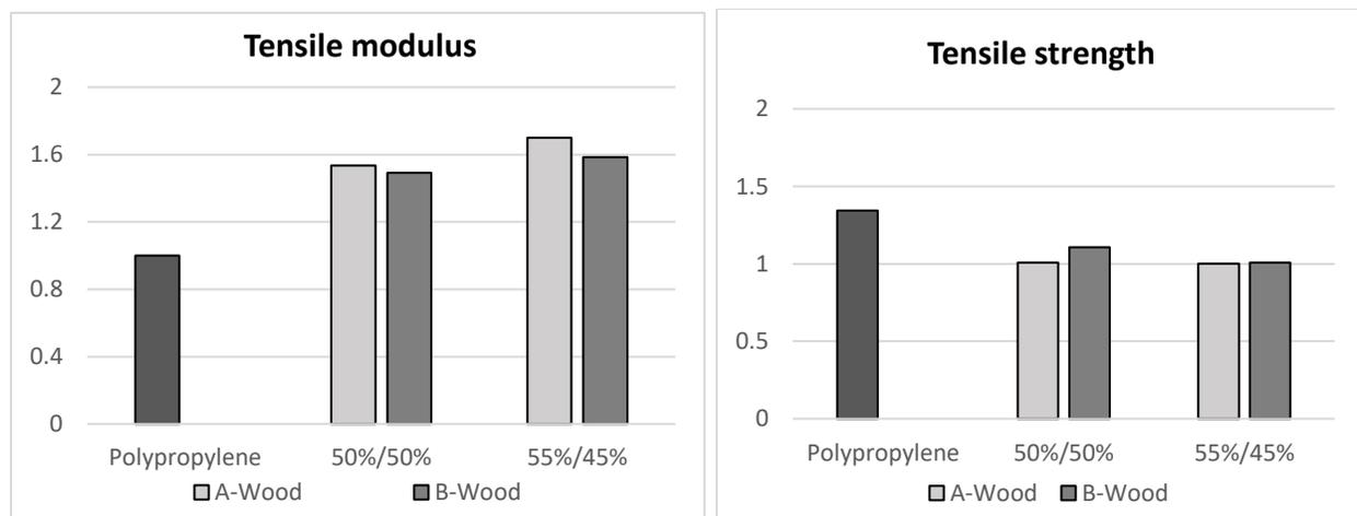
Figure 3. Tensile properties of wood fibre composites. The values are normalized with respect to the tensile modulus and strength of the matrix (PP).
