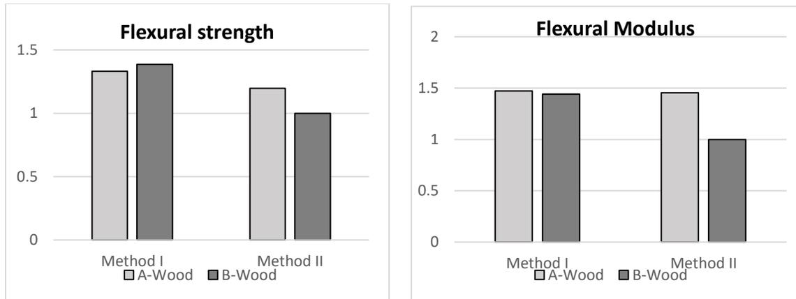
Figure 4. Effect of mixing on the flexural properties of wood fibre composites. The values are normalized with respect to the smaller value.
