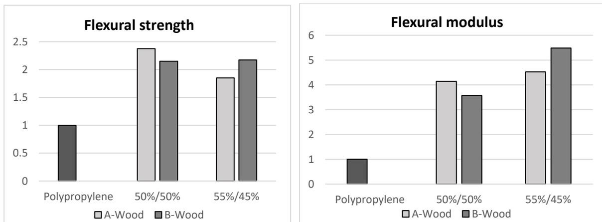
Figure 5. Flexural properties of wood fibre composites. The values are normalized with respect to the flexural modulus and strength of the matrix (PP).
